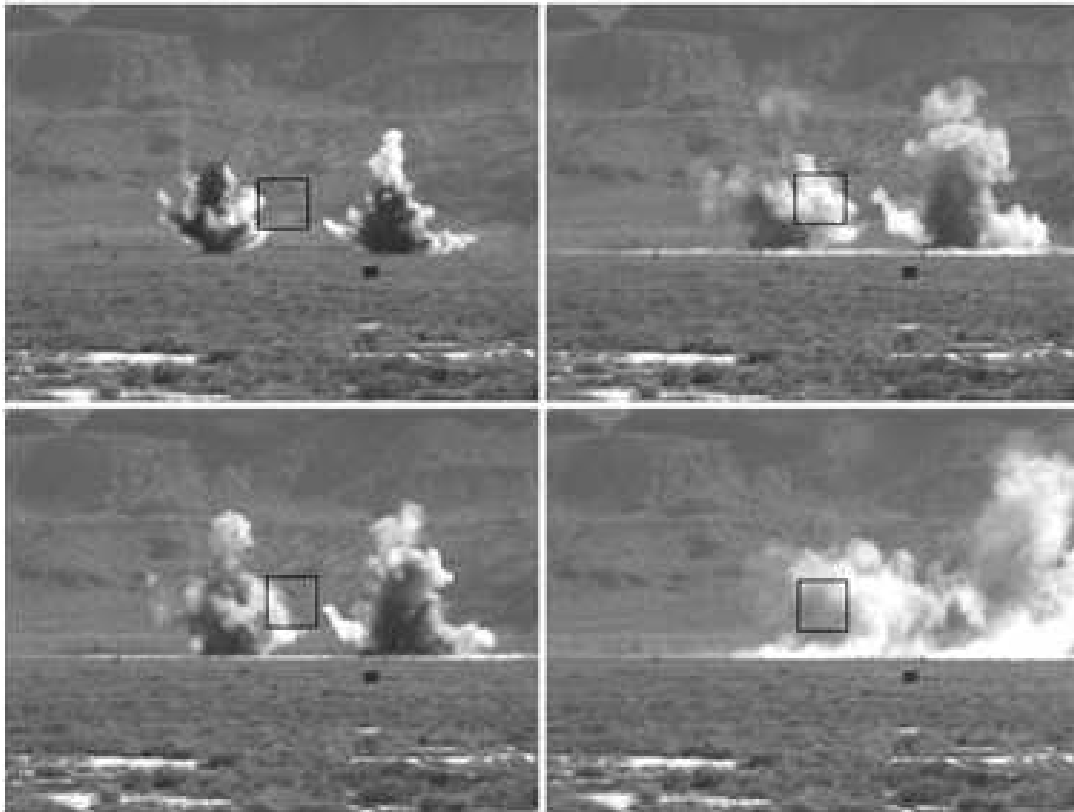
Figure 43. A series of LWIR thermal images of the explosive detonation release of MeS was acquired with the FLIR QWIP. Four such images are organized temporally from top left to bottom right. The black square within each image frame depicts the corresponding field-of-view of the FIRST-MWE visible camera, with telescope in place.
