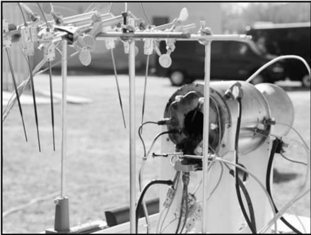
Figure 17. Rake of six k-type thermocouples to make in situ temperature measurements of the jet engine exhaust plume, viewed at an angle to portray locations of individual thermocouples with respect to the engine.
