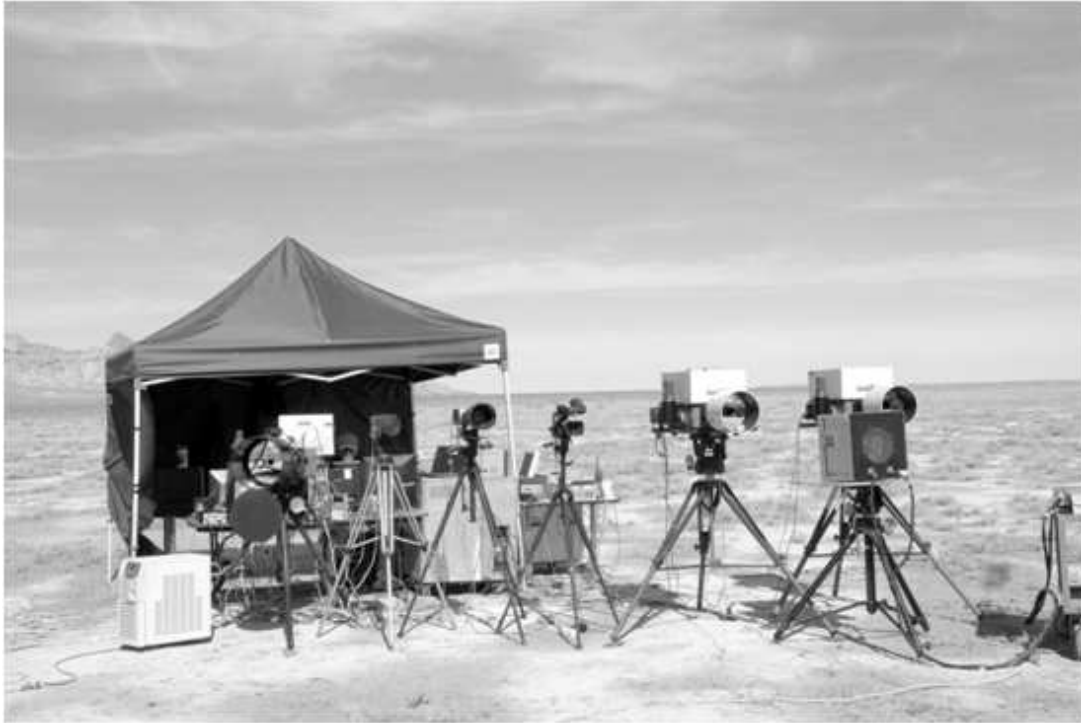
Figure 39. AFIT Remote Sensing team test setup at site 2. From left to right, the instruments used to collect test data: Telops FIRST-MWE, with optional telescope in place; FLIR QWIP Camera; Phantom camera; Canon camera; Bomem MR-254 FTS; Bomem MR-154 FTS. A water chiller to help cool the FIRST-MWE is located at the far left of the image, and a wide-area blackbody, used for FTS calibration, is located between the two Bomem spectrometers, to the right of the image. The instruments were monitored by a 3-person team from the control center of computer systems, shaded by the two-sided tent.
