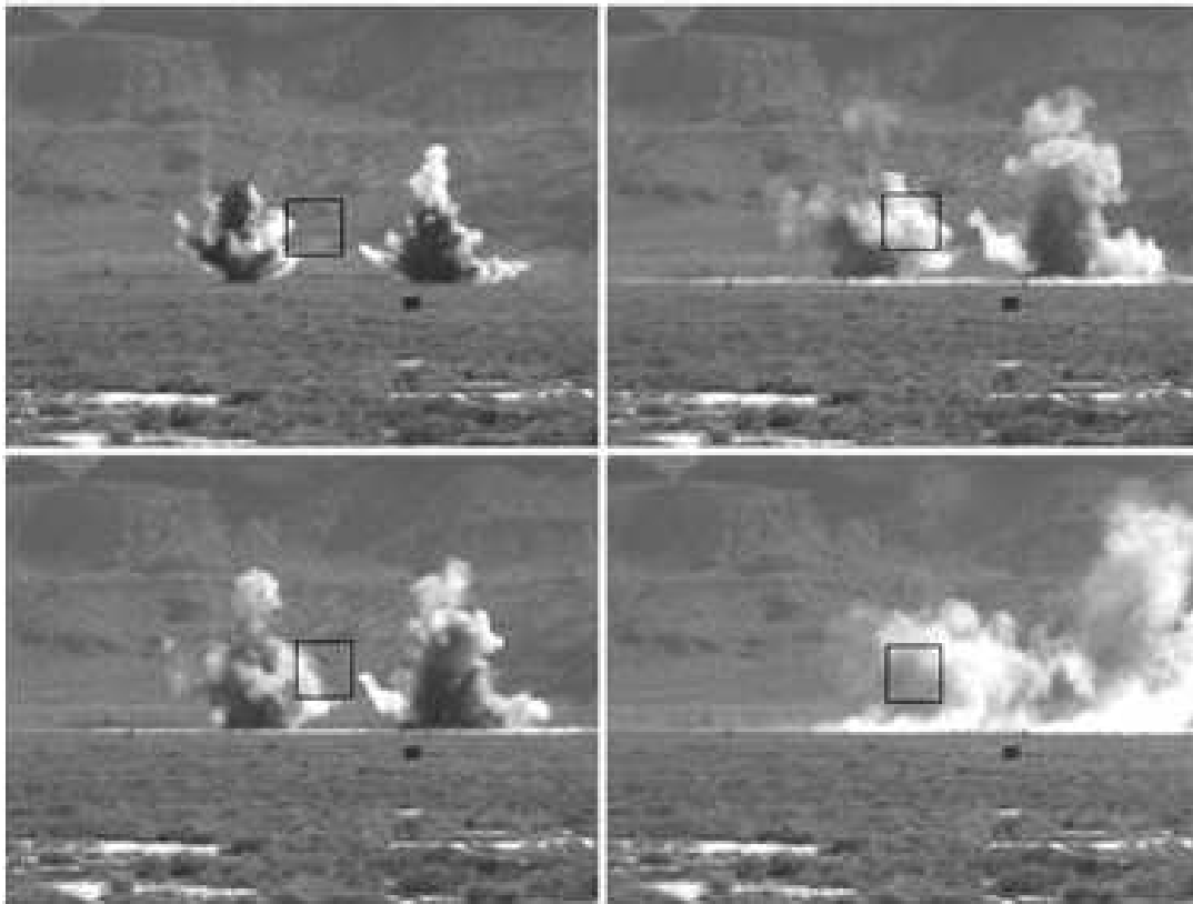
Figure 44. A series of images of the explosive detonation release of MeS was acquired with the FIRST-MWE boresighted visible camera, with telescope in place. Four such images are organized temporally from top left to bottom right. The black square within each image frame depicts the corresponding FOV of the FIRST-MWE imaging FTS.
