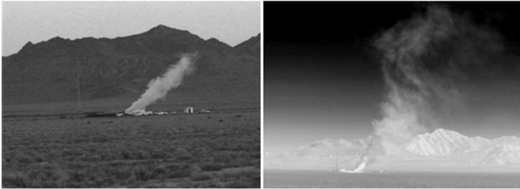
Figure 40. Non-mobile stack release of MeS. Left: Visible image acquired with the boresighted camera of the Telops FIRST-MWE during data collection, with telescope in place. Right: LWIR thermal image acquired by the FLIR QWIP camera during the same test event.
